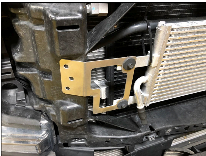
FIGURES 20 & 21 : Positioning The Cooler Using Cable Ties
