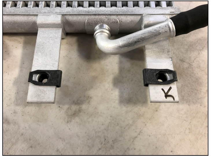
FIGURE 2 : Orientation of Capture Nuts
