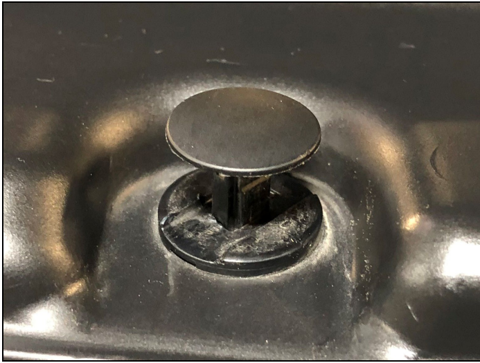
FIGURE 5 : Retainer Pin Popped Up
