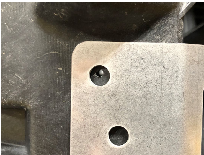
FIGURE 23 : Pre-Drill Hole Position
