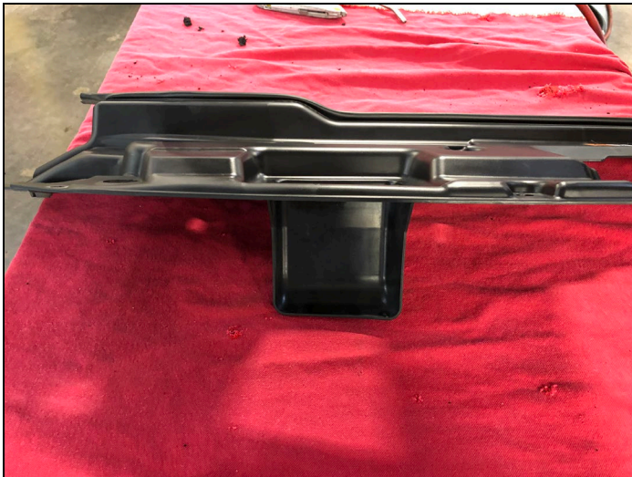
FIGURES 39 & 40 : Air Deflector Scoop – Before and After Trimming
