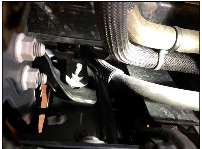
FIGURE 30 : Driver Side Hose Routing with Loom
