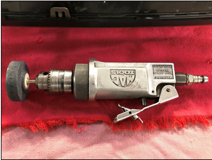
FIGURE 37 : High Speed Die Grinder with Grinding Stone
