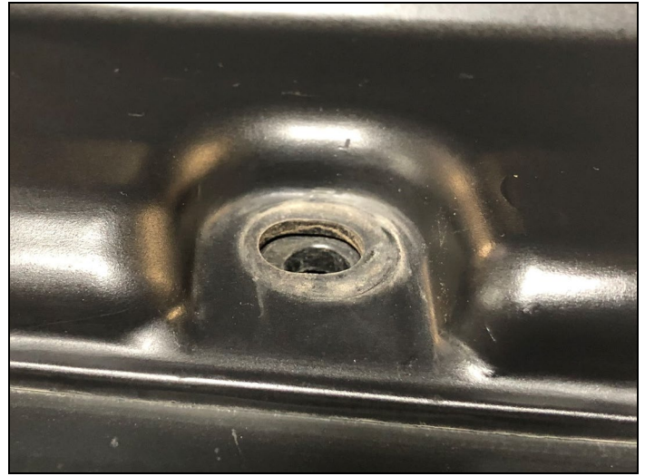
FIGURE 6 : Retainer Pin Removed
