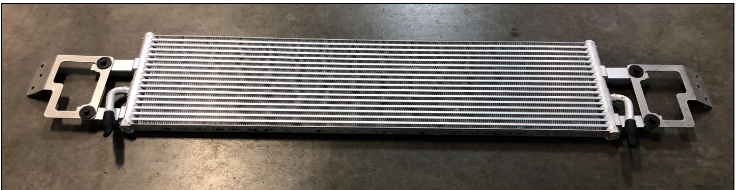
FIGURE 3 : Orientation of Installed Brackets – Note Direction of Bends and Orientation of Cooler Inlet/Outlet Tubes
