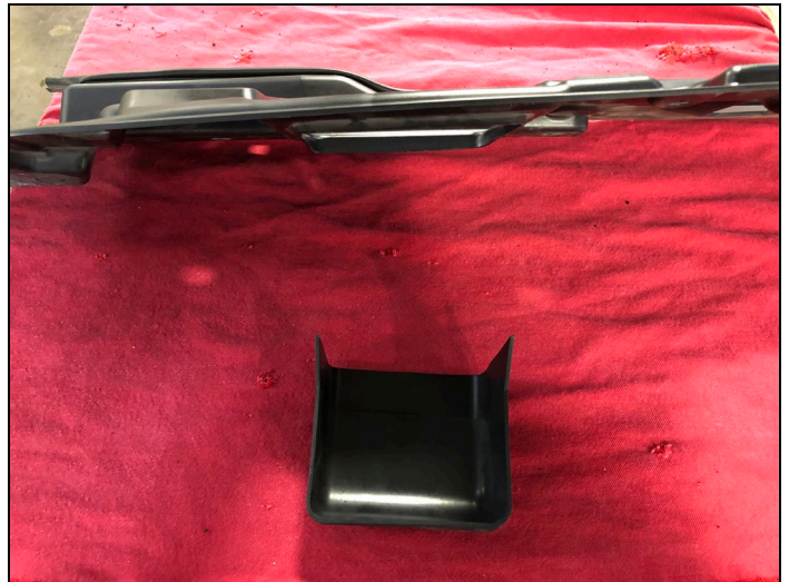
FIGURES 39 & 40 : Air Deflector Scoop – Before and After Trimming
