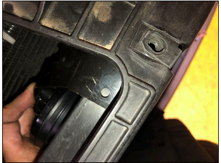
FIGURE 33 : Positioning Horn to Mark for Hole
