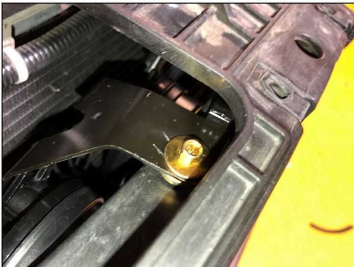
FIGURE 34 : Horn Installed w/Capture Nut, Spacer and Bolt
