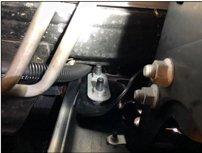
FIGURE 29 : Passenger Side Hose Routing with Loom
